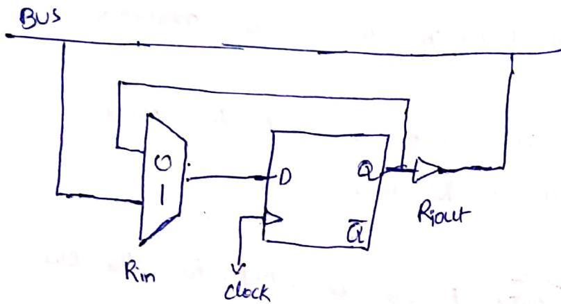
From the above diagram, Two input multiplexer is used. To select the data deployed to. The input of D flip-flop
